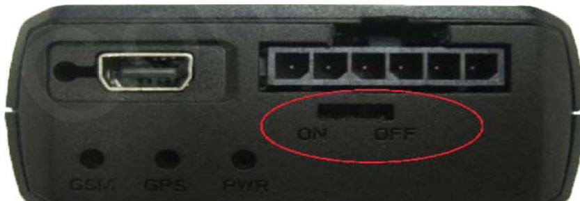
Figure 7. Switch and ON/OFF position
