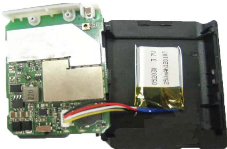
Figure 6. Backup Battery Installation
